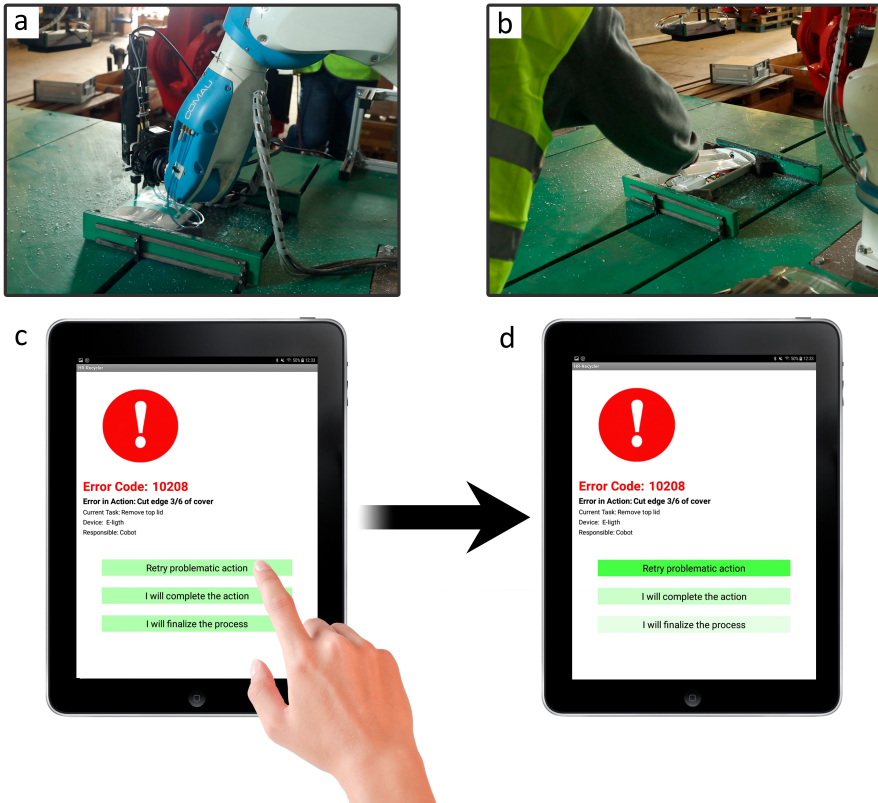
Figure 5.5. Personalized error-handling mechanisms during Human-Robot collaborative disassembly. a) The complex coupling of both the aCel and the DAC-HRC architecture becomes a potential source of failure that needs to be addressed at the systems level. b) Either when the cobot cannot complete a given disassembly action, or when is the worker's turn to execute a step of the disassembly, the human worker can intervene safely. c) IM app notification of an error during the disassembly providing the three different actions to overcome the error. d) The IM app in liaison with the Interaction Learner provides an attentional bias towards the preferred error-handling options by modulating their visual saliency.
