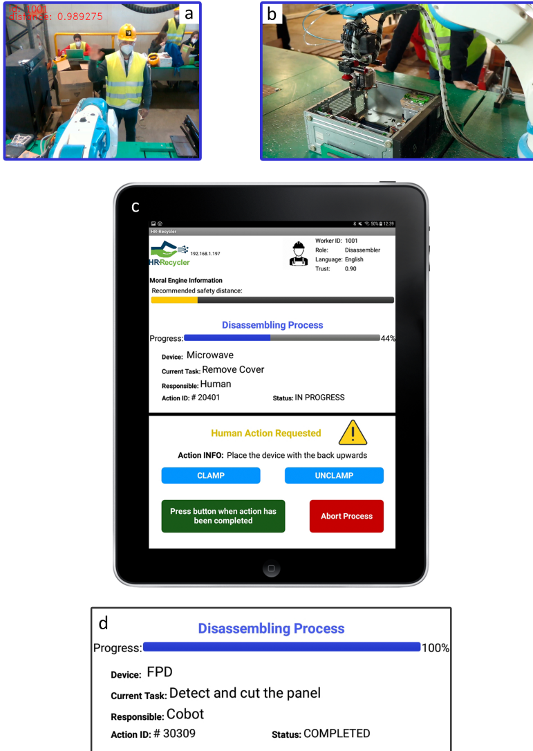
Figure 5.4. Human-Robot Collaborative Disassembly of a WEEE Device. (a) Vision module identifies a worker using their unique code. (b) DAC-HRC architecture adjusts to worker preferences, modulating robot behavior. (c) The IM app shows worker details and disassembly status, and sends notifications if human input is required. (d) Task Planner updates after full disassembly of the WEEE device.
